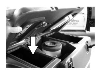
12. ES mode (option): When the solution tank has completely drained, replace the drain hose cap on the end of the solution tank drain hose. Place the solution tank draining hose on the lower retaining hook.
