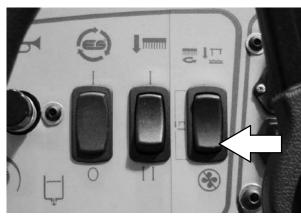
2. Press the top of the *one step switch* to start the normal scrubbing operations.
