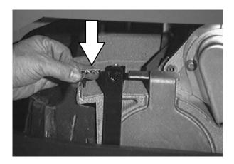
16. Cylindrical scrub head: Remove and clean the debris trough. Place the trough back in the scrub head when clean.
