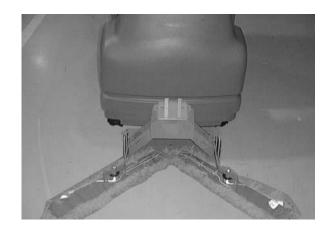
3. Connect the *QuickMop* attachment to the mounting bracket on the front of the machine.
