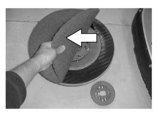
10. Replace the center disk to secure the pad in place on the driver.
