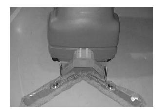
7. Remove and refasten the *QuickMop* head covers with the easy to remove snaps. Remove the head covers to rotate, shake and clean at regular intervals.
